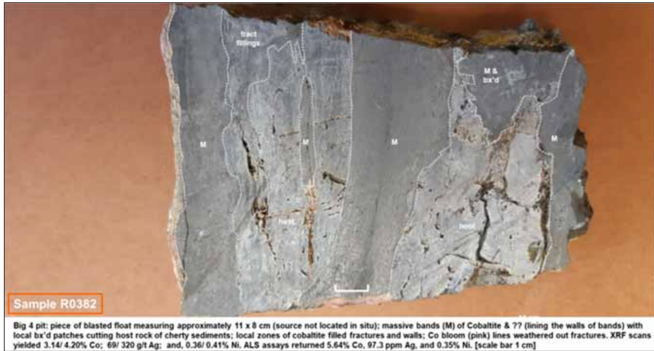
Figure 54: Cut Muck Sample of Cobaltite vein Showing the Internal Features.
