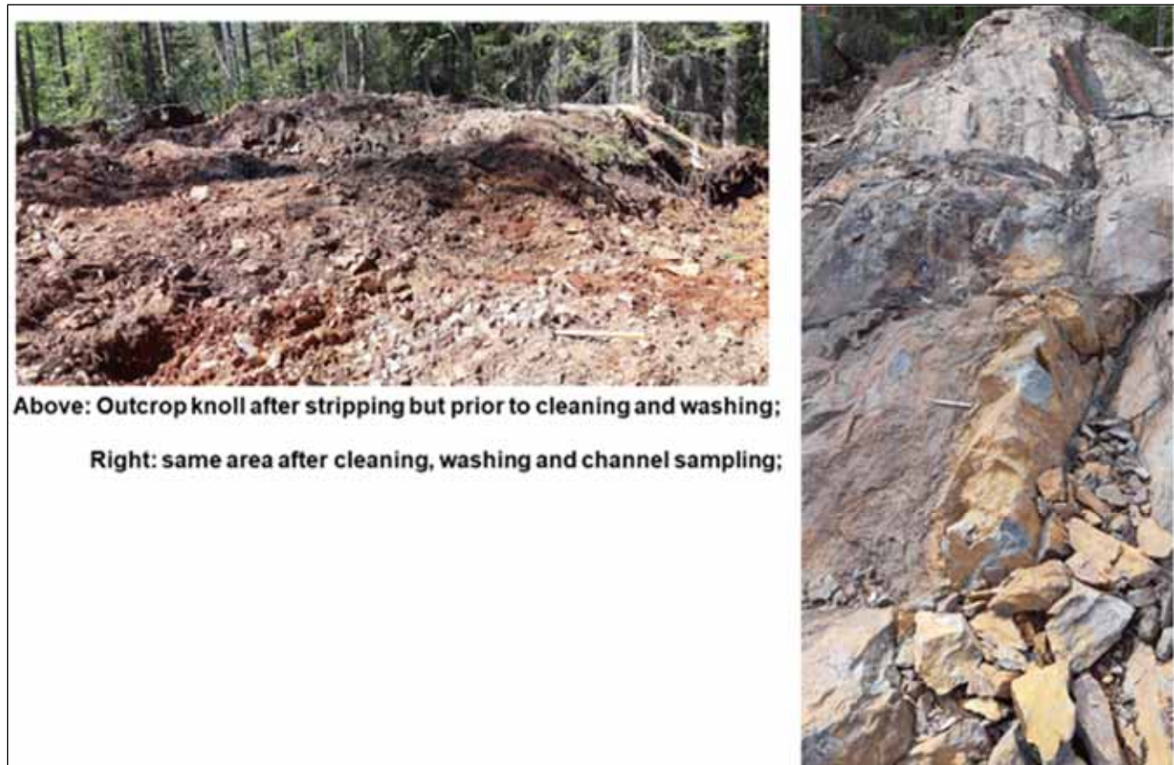
Figure 56: Before and After Cleaning Views of the Stripped Gossanous Knoll
