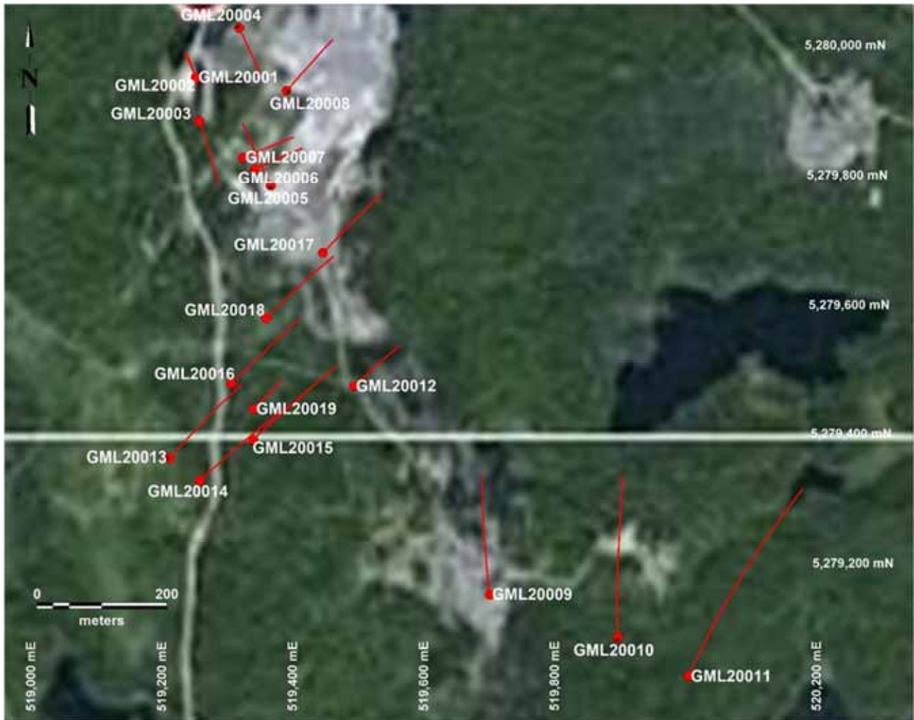
Figure 109: Gowganda-Miller Lake Target drill hole locations overlain on a satellite image (Google Earth)
