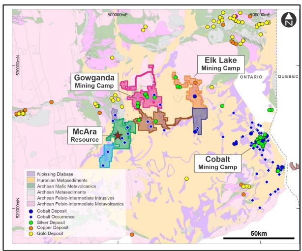
Figure 1: Cobalt Embayment Geology, BMR Claim Holdings and McAra Resource Location Plan
