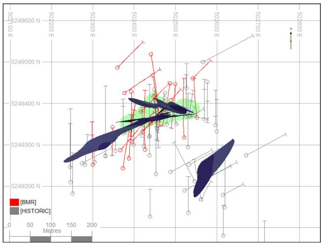
Figure 5: Distribution of Drillholes over the McAra Project Showing Modeled Mineralization Wireframes.
