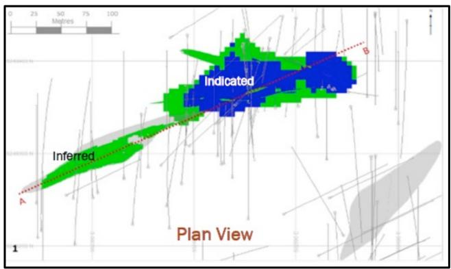
Figure 2: Mcara Mineral Resource Plan View Showing Informing Drilling - SRK Consulting (Canada) Inc. (2021)
