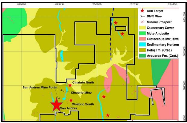
Figure 1: Punitaqui Geology with Deposits and Drill Targets
